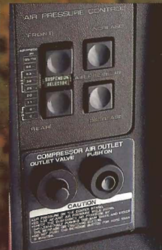
On-board air compressor.
